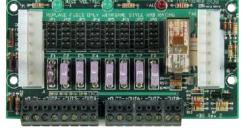
The Beacon multi-buss power distribution module is designed for use with AlarmSaf's Beacon Power Supply Line to provide flexible power management for access control system integration applications. There are two models available; the MB8F with 8 fuse protected outputs and the MB8 with 8 class 2, power limited outputs. Each output is individually selectable for FAI/egress control and output voltage. Ideal for use with all 8 or 16 door access control systems.
