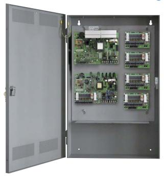
Dual Access Control Power Management System designed to supply regulated and filtered main, standby or auxiliary power to access system panels, door controllers, readers, ingress/egress security components, locking devices and auxiliary components. It will fully support up to 16 access controlled door locations.
