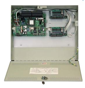
This unique multiple output power management system provides two separate outputs from a single 120 VAC input: **24 VDC, 6 Amp/ 12 VDC, 4 Amp, with 16 fuse protected outputs in a single cabinet** and will supply regulated and filtered main, standby or auxiliary power to access system panels, readers, ingress/egress security components, and locking devices.
