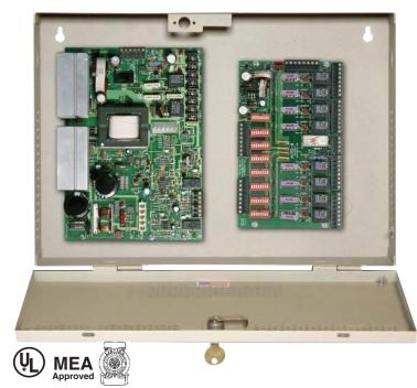
**12/24 VDC, 10 Amp** regulated power supply with advanced power distribution modules designed to manage power in access control and fire systems for full integration of life-safety building systems.
