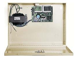
12/24 VDC, 10 amp switching power supply for access control and security systems integration. Features include field selectable voltage, Form "C" relay fault reporting, visual fault indication and an additional output for Fire Alarm Interface (FAI). Systems integration applications include system power, door strikes, mag locks, card readers and fire alarm interface for emergency exit.
