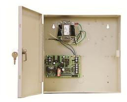
12/24 VDC, 4 amp switching power supply for access control and security systems integration. Features include field selectable voltage, power limited output, Form "C" relay fault reporting, visual fault indication and an additional output for Fire Alarm Interface (FAI). Systems integration applications include system power, door strikes, mag locks, card readers and fire alarm interface for emergency exit.
