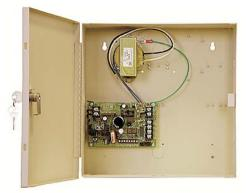
12/24 VDC, 2.5 amp switching power supply for access control and security systems integration. Features include field selectable voltage, power limited output, Form "C" relay fault reporting, visual fault indication and an additional output for Fire Alarm Interface (FAI). Systems integration applications include system power, door strikes, mag locks, card readers and fire alarm interface for emergency exit.
