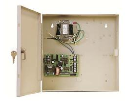
12/24 VDC, 4 amp switching power supply is agency listed for access control (UL 294 and CSA Certified). Features include field selectable voltage, power limited output, Form "C" relay fault reporting, visual fault indication and an additional output for Fire Alarm Interface (FAI). Systems integration applications include system power, door strikes, mag locks, card readers and fire alarm interface for emergency exit.
