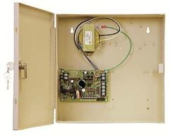
12/24 VDC, 2.5 amp switching power supply is agency listed for access control (UL 294 and CSA Certified). Features include field selectable voltage, power limited output, Form "C" relay fault reporting, visual fault indication and an additional output for Fire Alarm Interface (FAI). Systems integration applications include system power, door strikes, mag locks, card readers and fire alarm interface for emergency exit.
