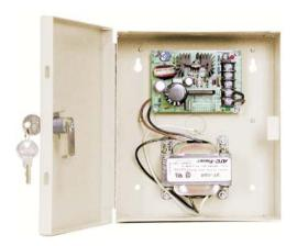
12/24 VDC, 2.5 amp (continuous) commercial switching power supply for systems integration featuring field selectable voltage, power limited output and visual fault indication. Common access control and security system applications include system power, door strikes, mag locks, card readers and other accessory devices.
