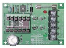
6/12/24 VDC, 1 amp (continuous) commercial power supply for systems integration featuring field selectable voltage and visual fault indication. Common access control and security system applications include door strikes, mag locks, card readers and other accessory devices.
