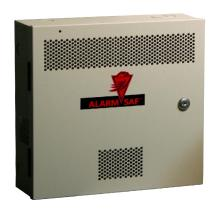
12 VDC, 1.5 Amp power supply with 14 Ah battery charge capacity for powering access control systems and auxiliary devices. The power supply includes a class 2, transformer and is supplied in a vented, steel, key lockable enclosure with space for a 14 Ah battery set.
