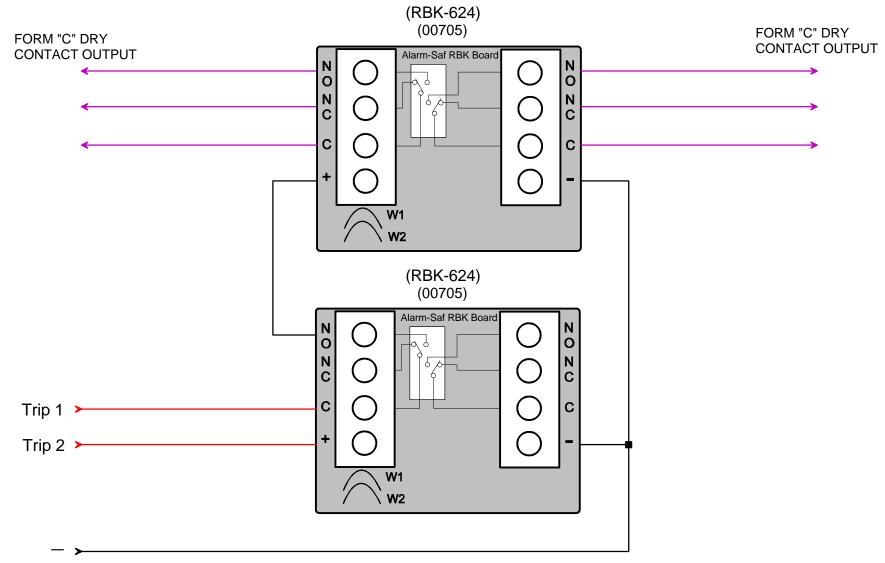
Application: For use when two seperate positive trip signals are required to activate a relay. The relay will activate only by applying a positive trip signal to both the + terminal and the C terminal of the RBK-624.
