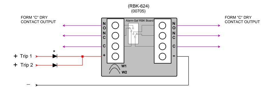
Application: For use when two seperate positive trip signals are needed to activate a relay. The relay will activate by applying one or two positive trip signals to the + terminal of the RBK-624.
