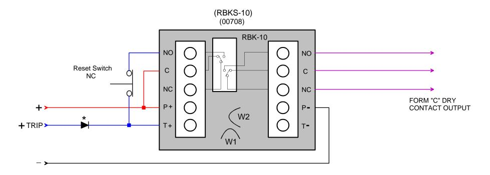
Upon application of a positive trip signal to the T+ terminal of the RBKS-10 the relay contacts transfer applying a positive voltage to the T+ terminal thus latching the relay in the alarm condition.
