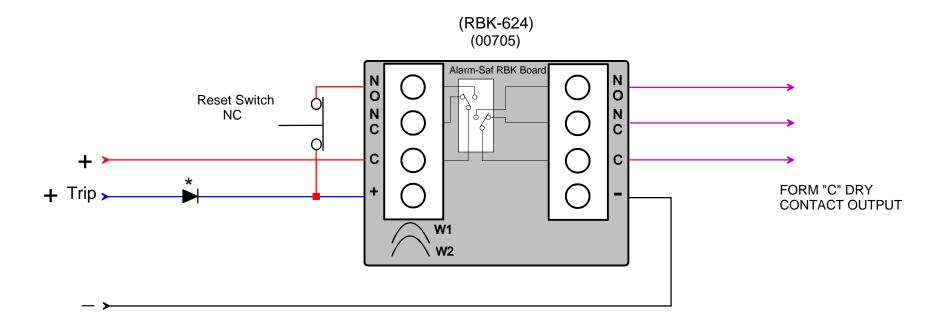
Upon application of a positive trip signal to the + terminal of the RBK-624 the relay contacts transfer applying a positive voltage to the + terminal thus latching the relay in the alarm condition.
