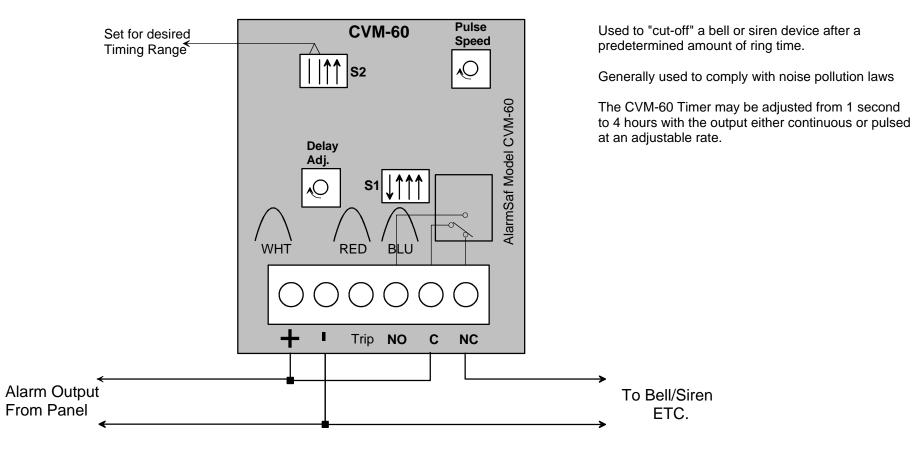
The CVM-60 Timer may be adjusted from 1 second to 4 hours with the output either continuous or pusled at an adjustable rate.
