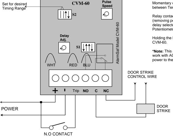
Momentary closure of normally open contacts connected between Terminal 1 and 3 will initiate timer operation.
